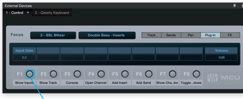
*Right-click on the button and click 'Assign Command...' to change the function of any of the F keys.*
